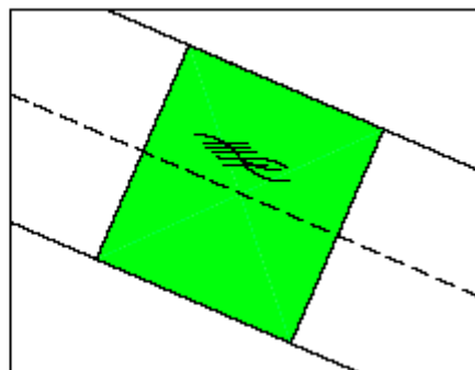
Figure 10: Damaged pavement within 10 feet of a patch must also be patched.
